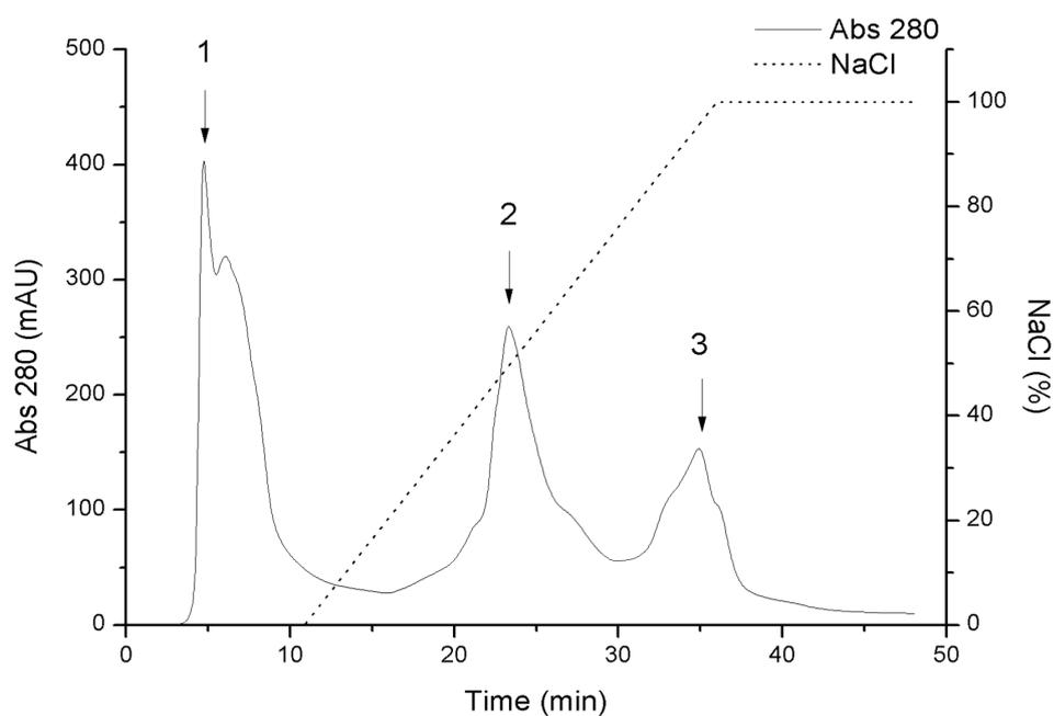
**Figure 6.** Anion exchange chromatography (Q-Sepharose High Performance) of EE. Column diameter: 1.6 cm; column height: 16.5 cm; starting buffer: Tris-HCl 50 mM, pH 8.5; elution saline gradient: 165 mL of 0.0–0.1 M of sodium chloride in the starting buffer. Flow rate, 1.0 mL min<sup>-1</sup>. The arrows indicate proteolytic activity in the unretained fraction (peak 1) and retained fractions (peaks 2 and 3).
