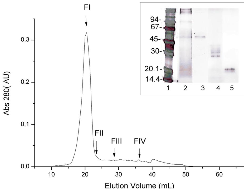
**Figure 7.** Size exclusion chromatography with Sephadex G-75. Fractions of 0,5 mL were collected at a flow rate of 0.250 mL/min and analyzed at 280 nm. The arrows indicate proteolytic activity in fraction I (FI), II (FII), III (FIII) and IV (FIV). Inset to Fig 7. SDS-PAGE of the fractions with proteolytic activity FI (lane 2), FII (lane 3), FIII (lane 4), FIV (lane 5) and the molecular weight standard (lane 1).
