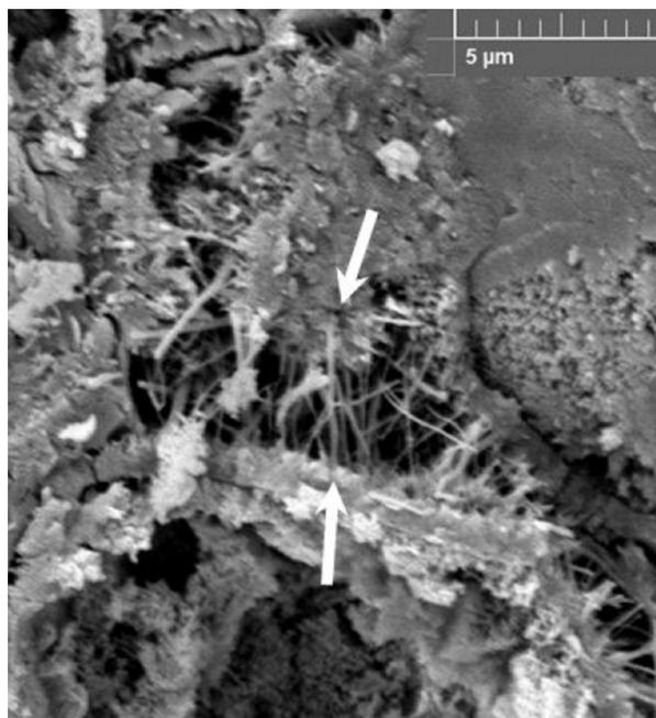
**Figure 9.** Micrograph of the failure surface of [PM+SNF+MWCNT] sample. The arrows indicate the links of MWCNT with the matrix material.
