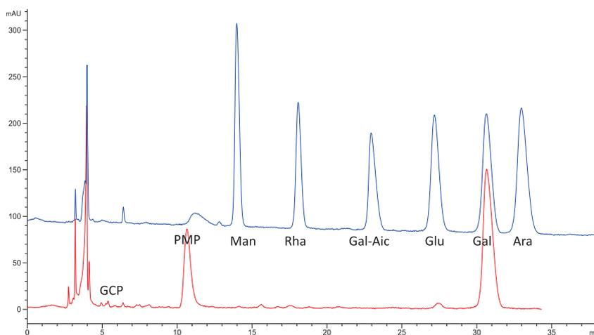
**Figure 3** - HPLC chromatogram of monosaccharide composition of GCP.
