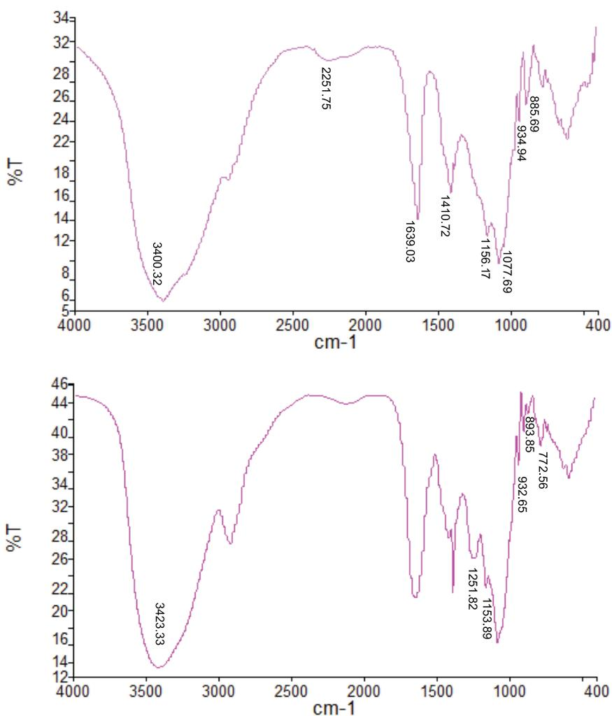
Figure 5 - FT-IR spectrum of GCP-1 and GCP-2.
