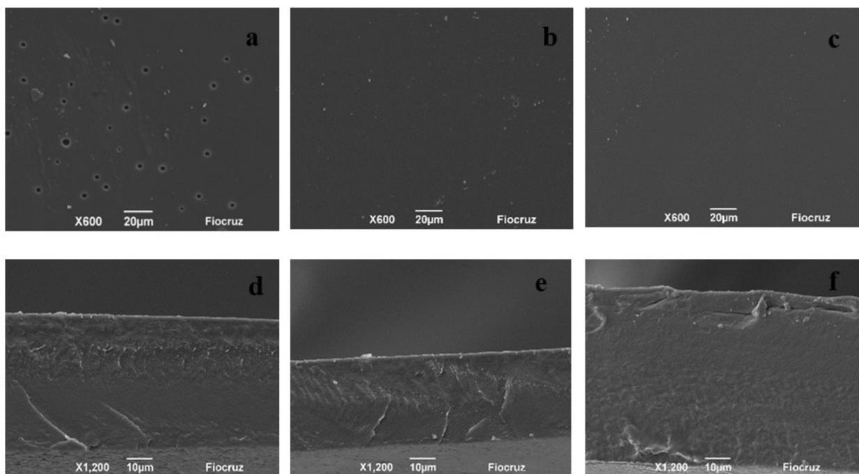
**Figure 1.** Surface (top) and cross-sectional (bottom) scanning electron microscopy (SEM) images of PBAT films produced by casting: OE00.0 (left; a and d), OE05.0 (middle; b and e), and OE07.5 (right; c and f).
