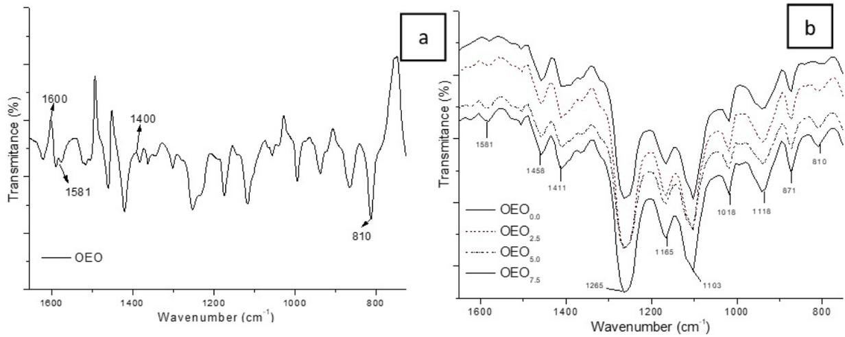
Figure 3. FTIR spectra of PBAT films incorporated with different OEO concentrations: (a) OEO and (b) OEO0.0 to OEO7.5.”
