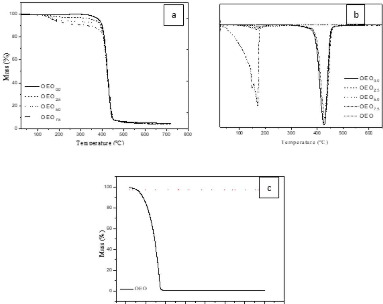
Figure 4. Curves of TGA (a and c) and DTG (b) OEO and formulated films.”
