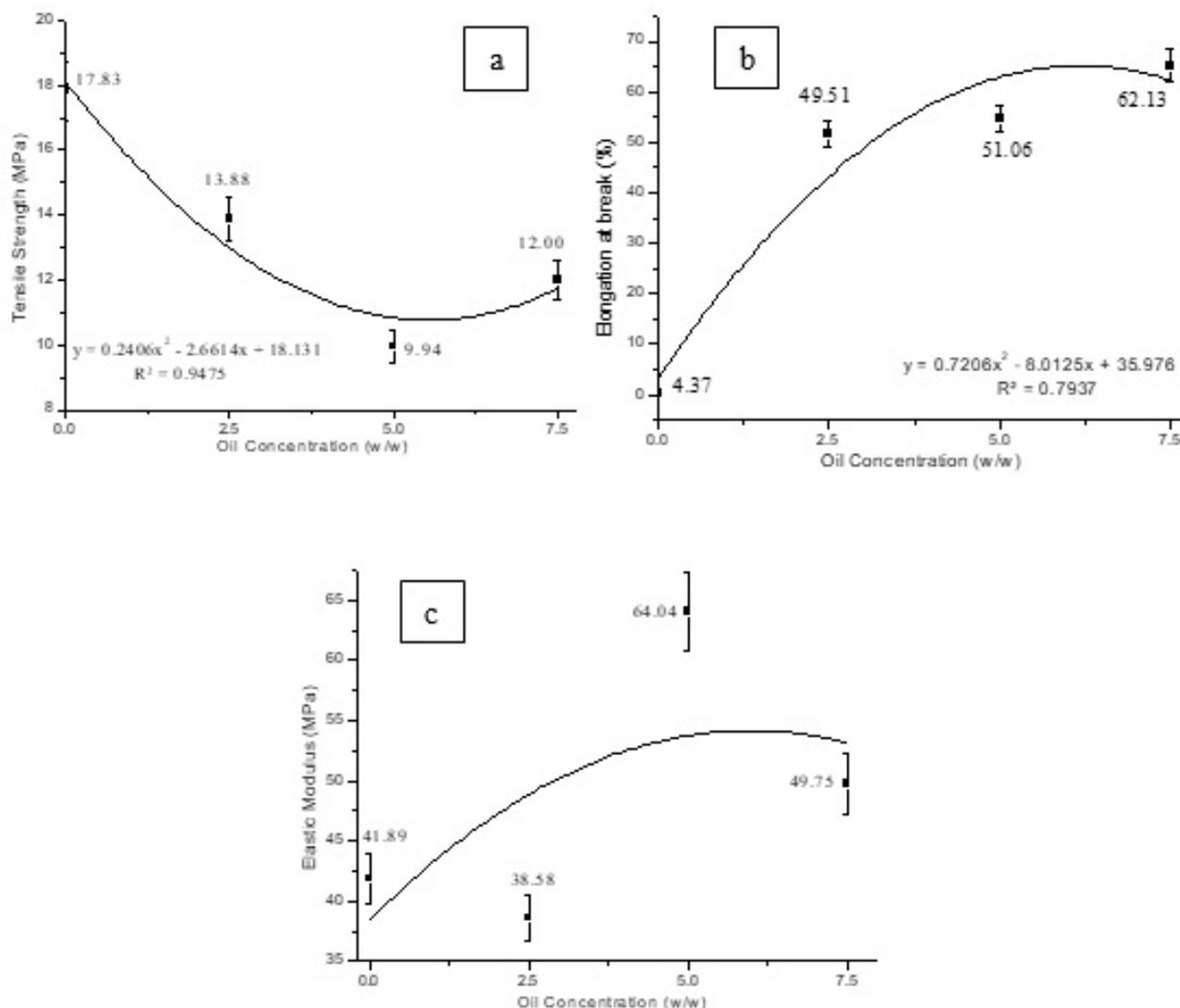
**Figure 2.** Mechanical properties of PBAT films produced by casting, where axis x = oil concentration (g) and axis y = (a) maximum strain; (b) elongation at break, and (c) elastic modulus.
