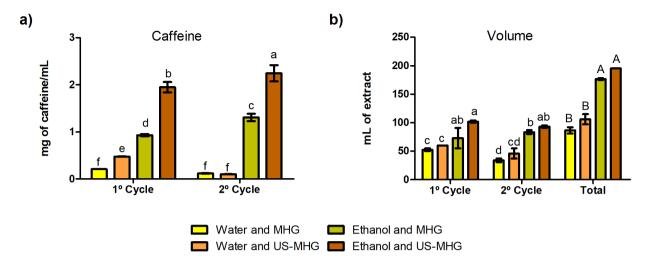
**Figure 1.** Influence of solvent, ultrasound pretreatment, and the number of cycles on the extraction of caffeine from guarana powder; a) caffeine concentration in guarana extracts; b) volume of extract. The samples from the first and second cycles followed by at least the same lower-case letter do not differ from each other by the Duncan test (p> 0.05). The samples of the total volume of extract followed by the same capital letter do not differ by Duncan test (p> 0.05).
